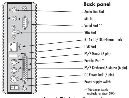
Figure 6. Thin System - Back panel
